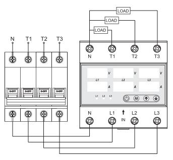
Rated operating current of circuit breaker is 75% maximum current of the relay le=0.75x lmax
